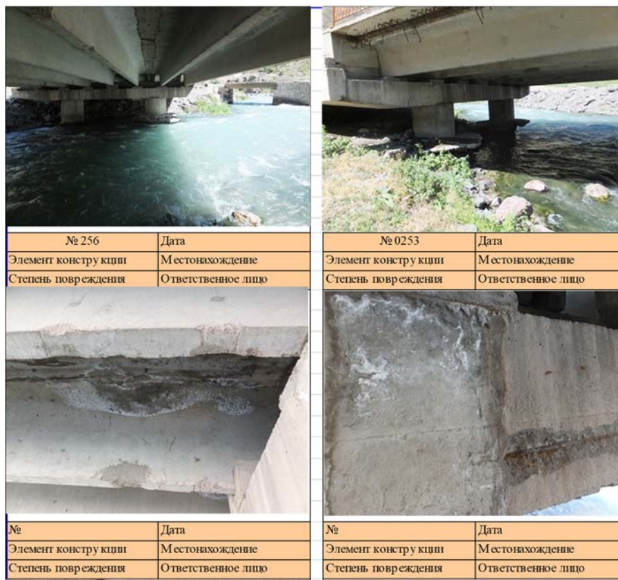
Figure 2-3 Bridge Inspection Format of Planned Inspection A
