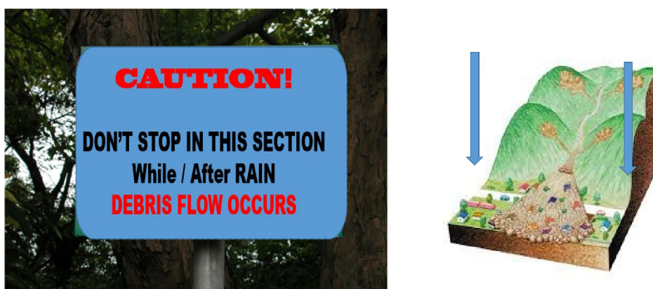
Figure 10.3-9 Installation image of sign board to prevent involvement in debris flow
