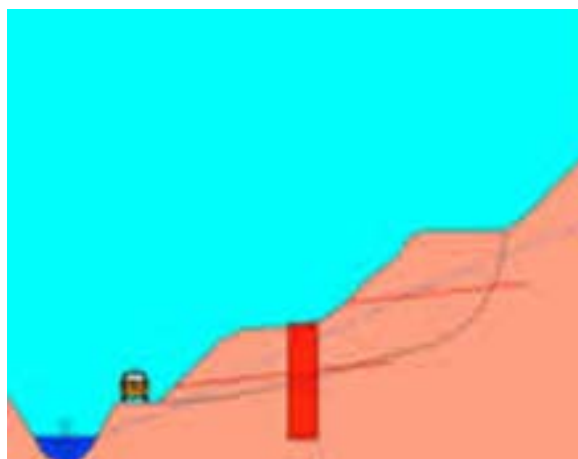
Figure 4.3-8 Shaft Work for Landslide
