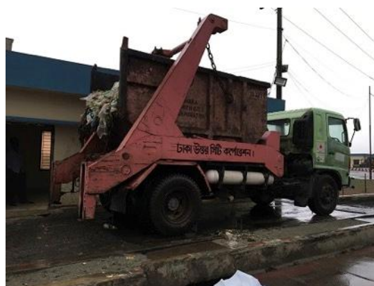
Photo 2: Container carrier of DNCC on a truck scale of the final disposal site
