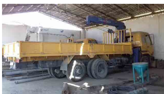
Procured crane-mounted truck
