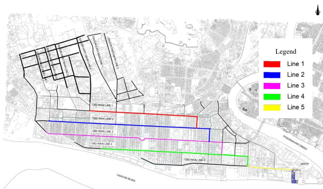
Figure 6.8.5 Detail of Proposed Sewer to Be Installed in CBD with BDS
