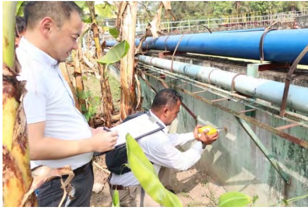
Photo 3: Concrete Chipping Survey (Reactor of C1 WWTP) Figure 1: Schmidt Hammer
