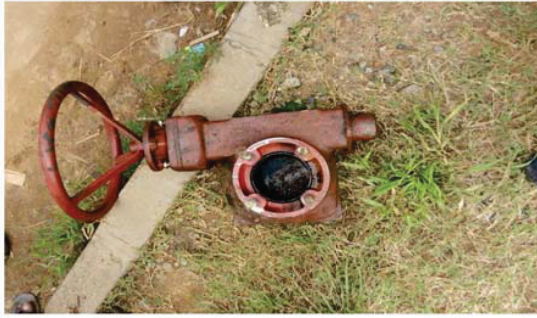
REPLACEMENT OF FAILED BUTTERFLY VALVE D500MM AT NYANYAN
