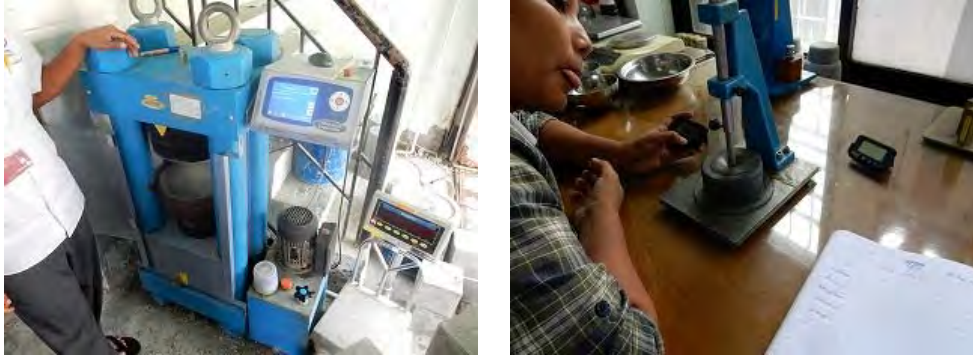
Figure 3.3.11: (Left) Concrete Compression Test, (Right) Consistency Test
