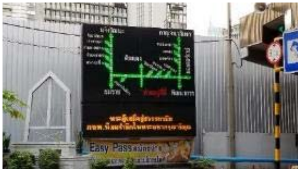
ITS system : VMS at Nana
