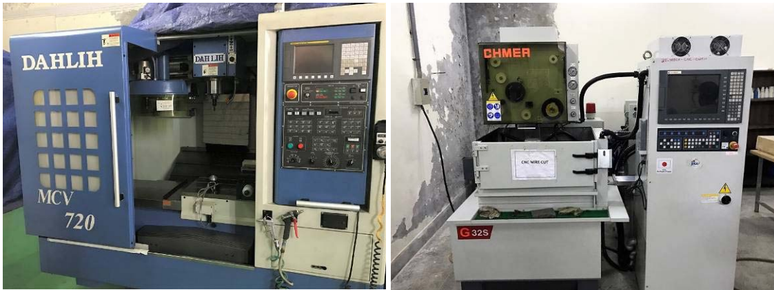
CNC processing machines of the Architecture Department (for practical training)
