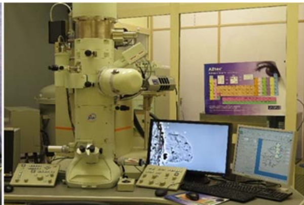
Transmission electron microscopy used for analysis of microscopic regions of engineering materials etc.
