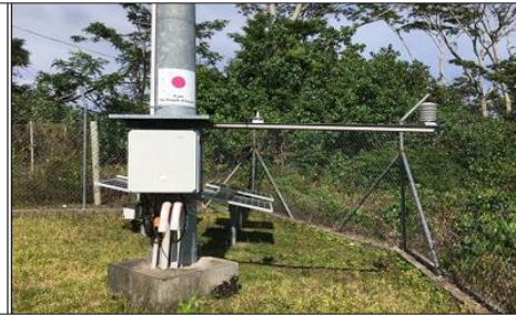
Data Collection Unit, Barometer, Temperature and Humidity Sensor (Le Piu Tai in Savaii Island)
