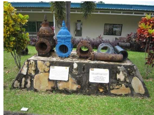
Rusted water distribution pipe replaced in the Project and model of newly installed water distribution pipe (Preah Sihanouk)
