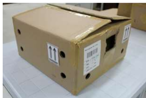
BC flute corrugated fiberboard box with cross partition
