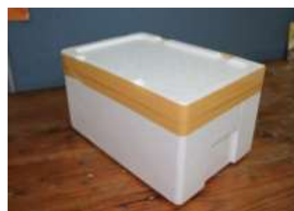
Hand-carrying box (2): Fillet Box 40 times expanded EPS foam box L320 × W200 × H140mm, T: 20mm
