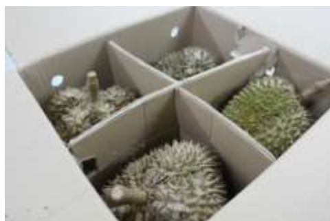
BC flute corrugated fiberboard box with cross partition
