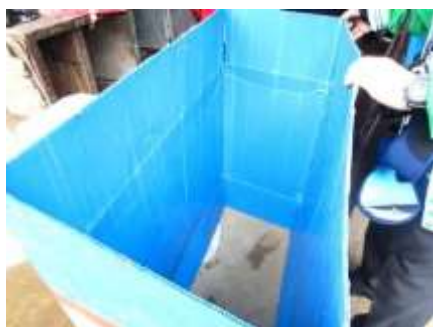
Returnable corrugated plastic box (310 pesos/piece, durable for 8-10 times of use) W 100 cm x H 60 cm x L 45 cm Shipping cost: 140 pesos/box
