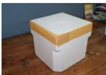
Hand-carrying box (2): Fillet Box 40 times expanded EPS foam box L320 × W200 × H140mm, T: 20mm
