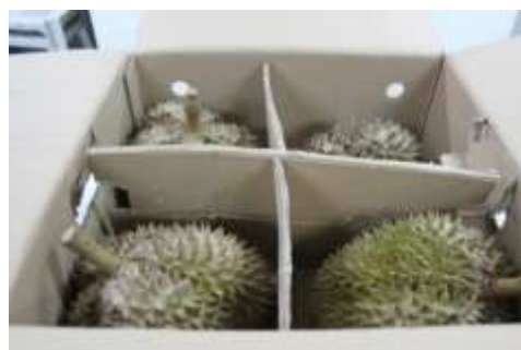
BC flute corrugated fiberboard box with cross partition
