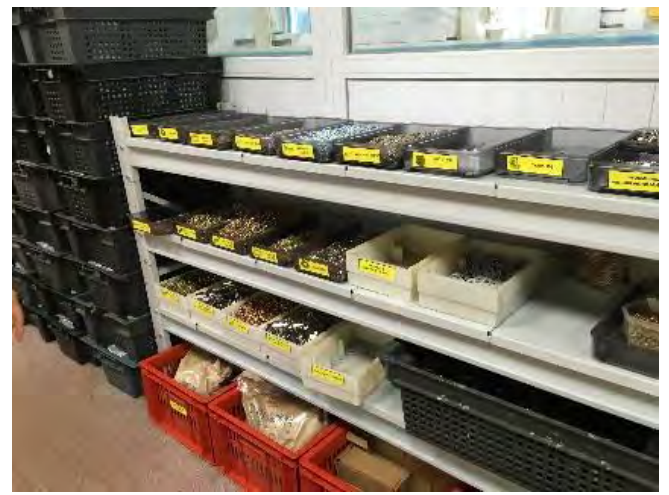
Parts organized based on kaizen principles so that the remaining volume is visible at a glance (at a company whose staff participated in the business course)
