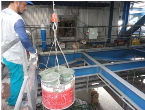
A Staff Bringing Combustion Mediator (Silica Sand) which is Used for CFB Boiler
