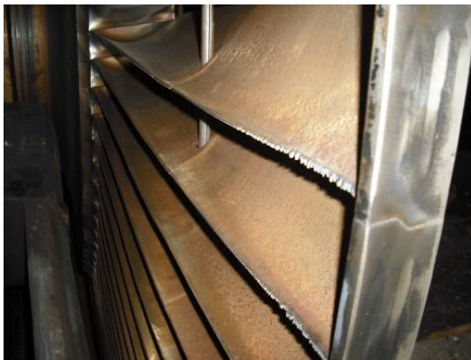
Fig.4.2-16 LP Last Blade before Repair
