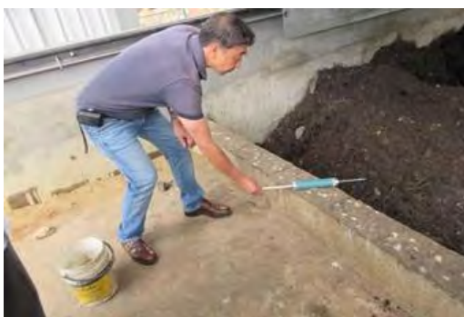
Picture 12 Measurement with Kitagawa type detection tube
