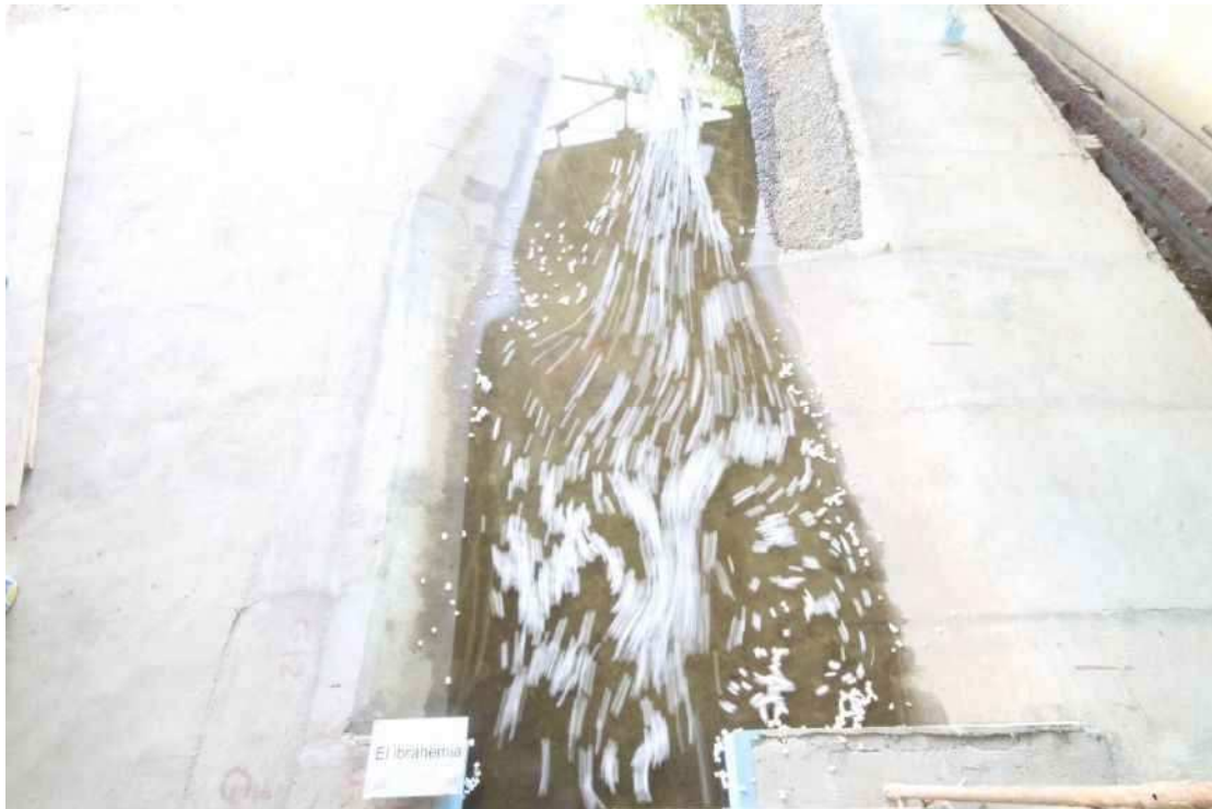
Photo 13: Flow Tracking Downstream New Ibrahimia Regulator Using Floating Debris
