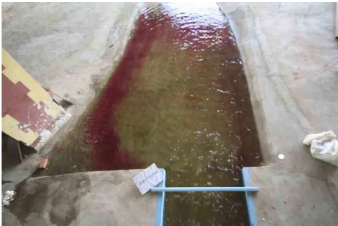
Photo 8: Flow Tracking Downstream New Bahr Yusef Regulator Using Colored Dye
