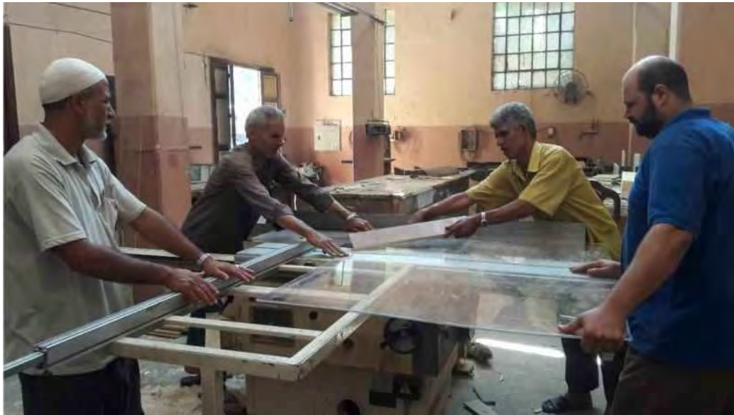
Plate (2A) Cutting the Plexiglas of the Half Pier
