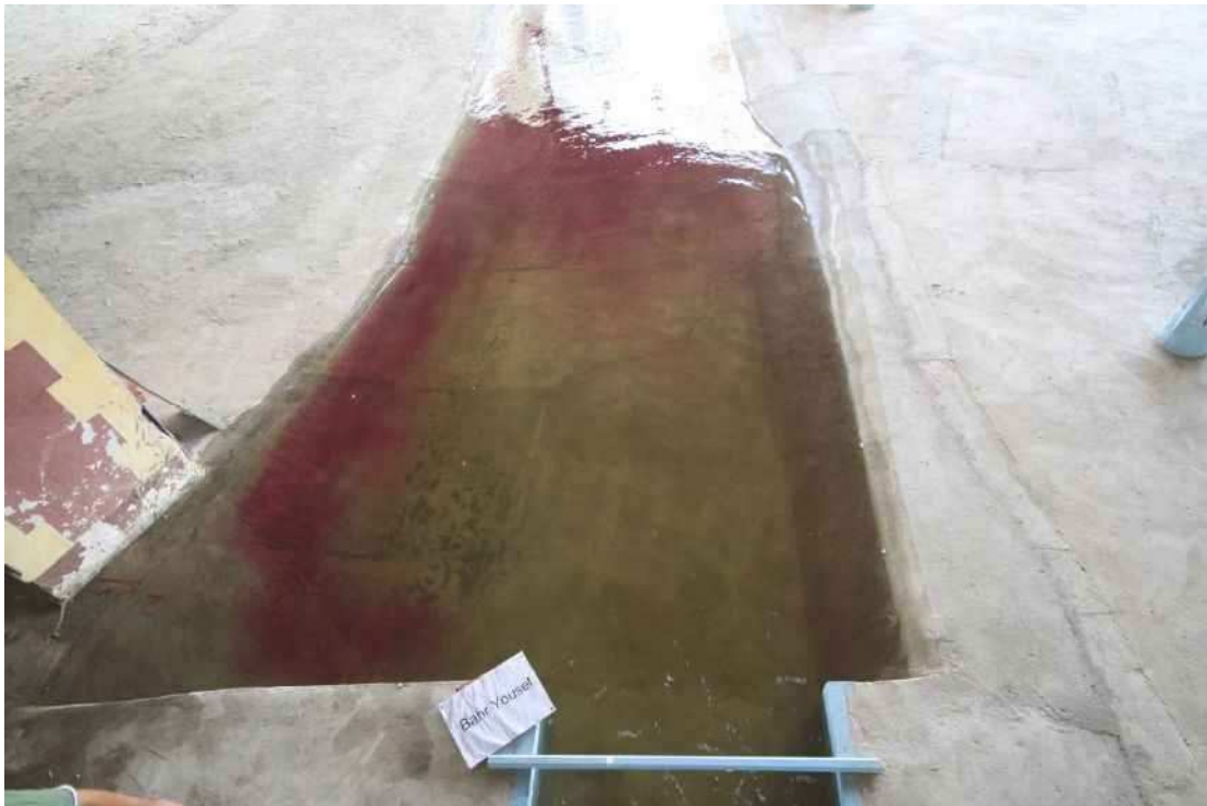
Photo 16 : Flow Tracking Downstream New Bahr Yusef Regulator Using Colored Dye
