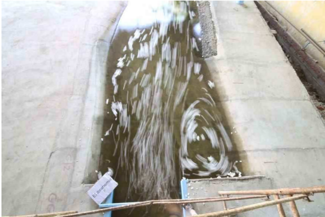
Photo 9: Flow Tracking Downstream New Ibrahimia Regulator Using Floating Debris
