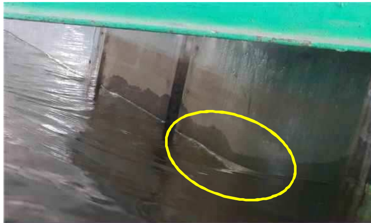
Plate 4.1 Drop of Water around Pier, Test-17
