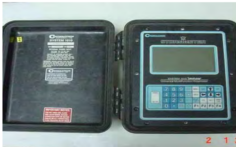
Plate (23): Ultra-Sonic Flow-meter Gauge
