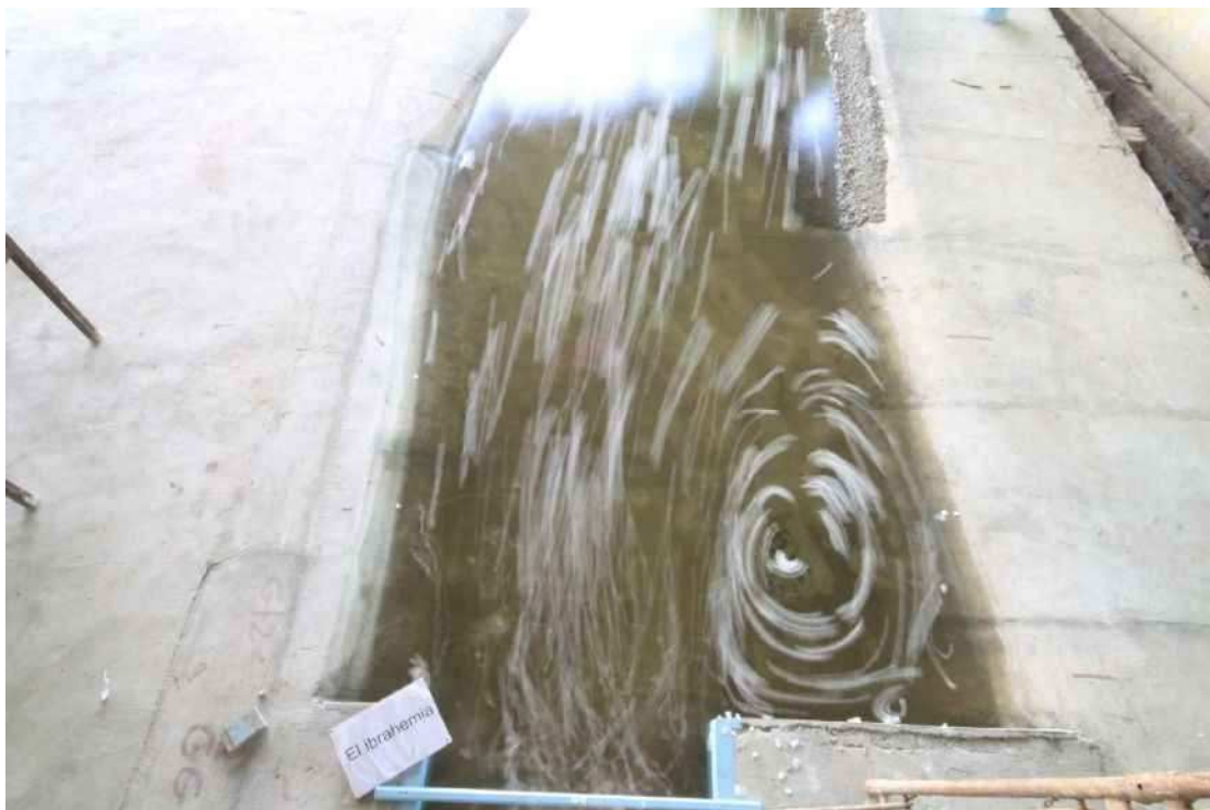
Photo 17: Flow Tracking Downstream New Ibrahimia Regulator Using Floating Debris
