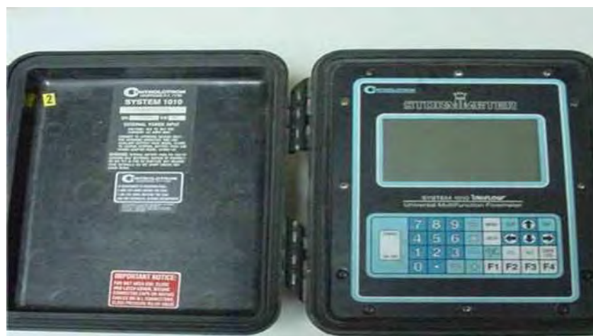
Plate (5) Ultra-Sonic Flowmeter for Inflow Discharge to the Model
