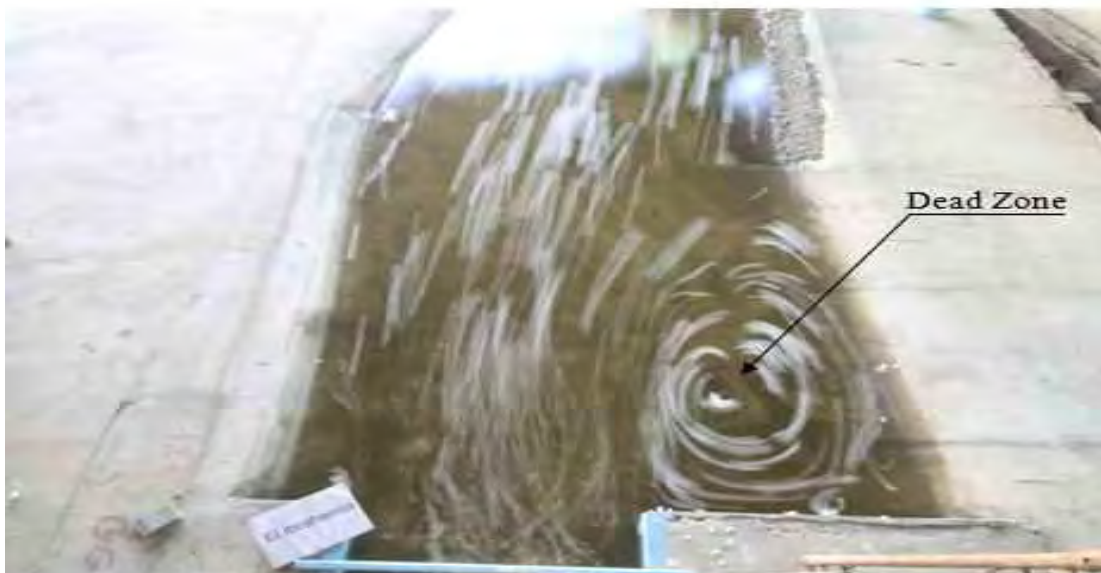
Figure (13): Formation of Dead Zone Downstream Ibrahimia New Regulator
