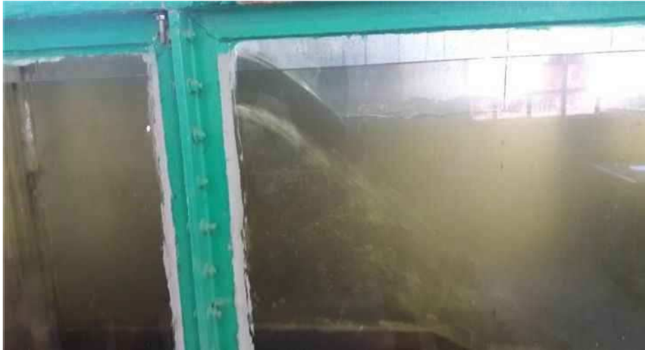
Plate (3.1) Show the Flow over the Gate, case -1
