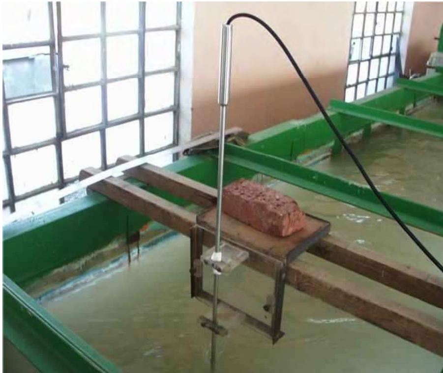
Plate (6) Electro-Magnetic Currentmeter for Velocity Measurements in the Model
