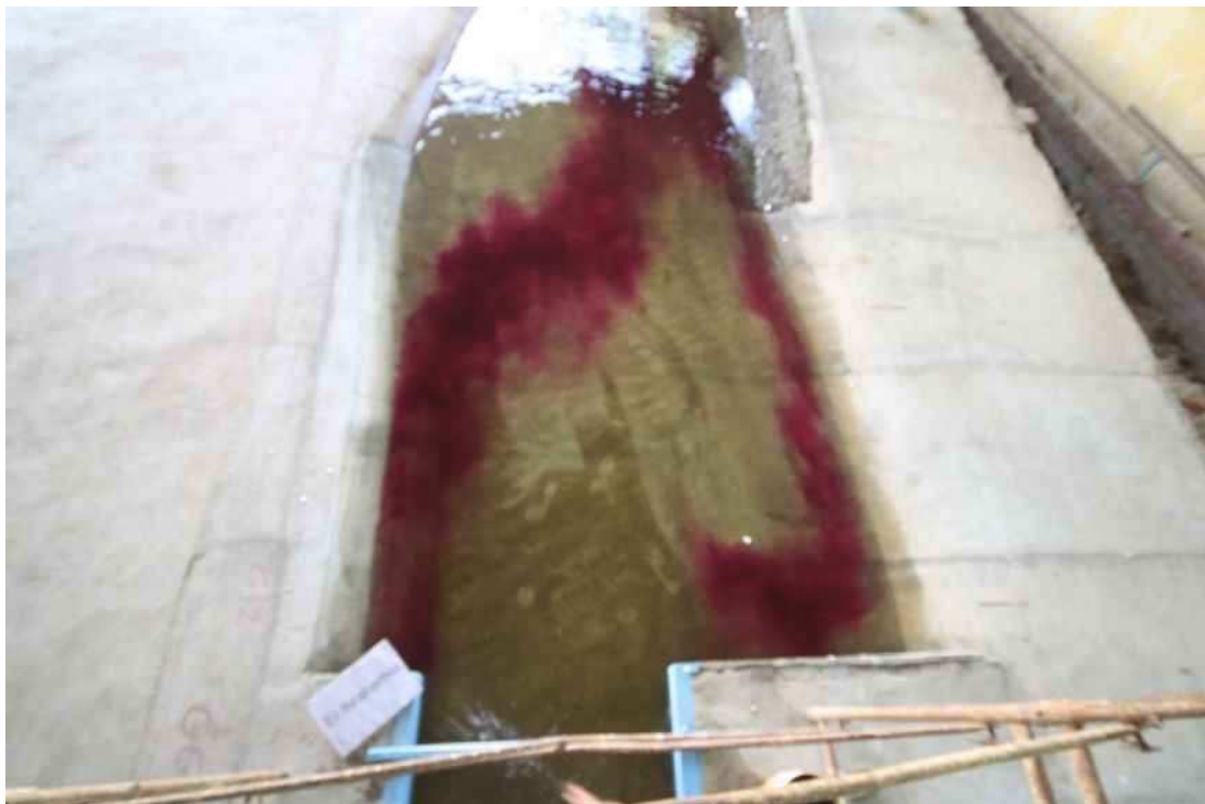
Photo 10: Flow Tracking Downstream New Ibrahimia Regulator Using Colored Dye
