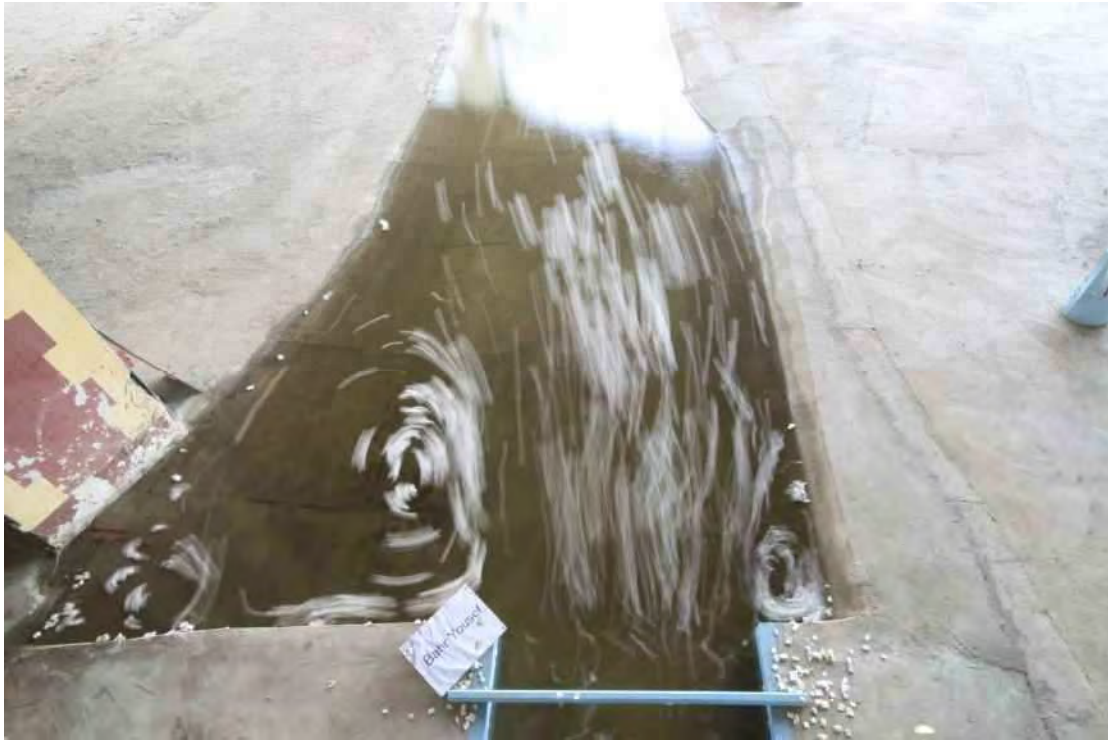
Photo 15: Flow Tracking Downstream New Bahr Yusef Regulator Using Floating Debris
