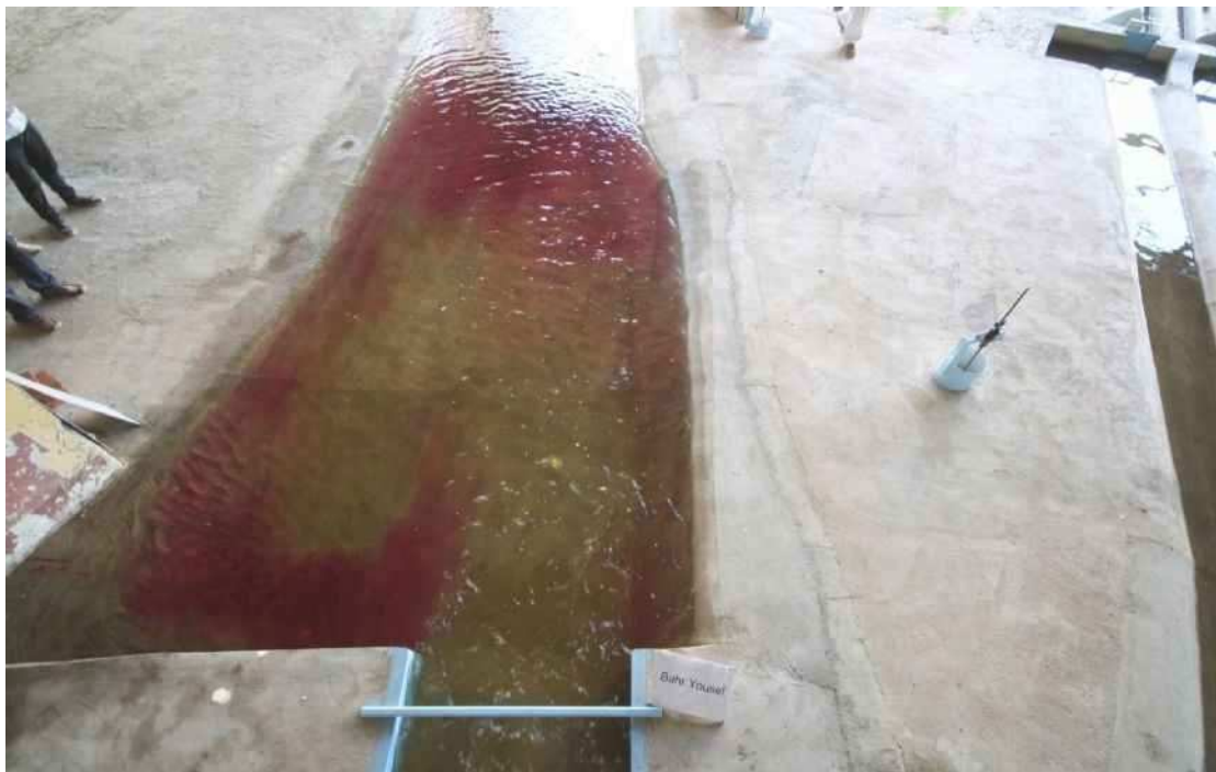
Photo 4: Flow Tracking Downstream New Bahr Yusef Regulator Using Colored Dye
