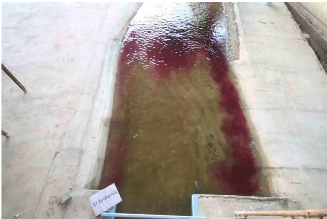
Photo 18: Flow Tracking Downstream New Ibrahimia Regulator Using Colored Dye
