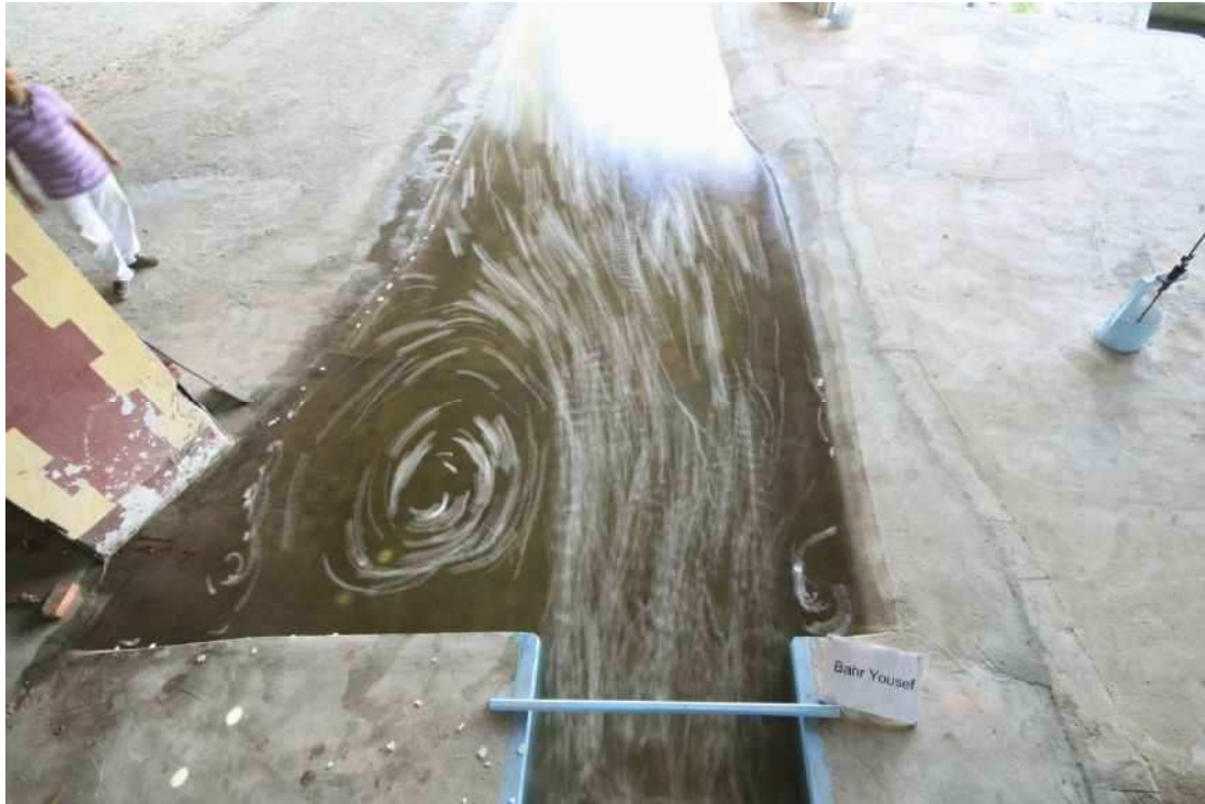
Photo 3: Flow Tracking Downstream New Bahr Yusef Regulator Using Floating Debris
