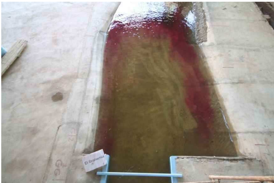
Photo 6: Flow Tracking Downstream New Ibrahimia Regulator Using Colored Dye
