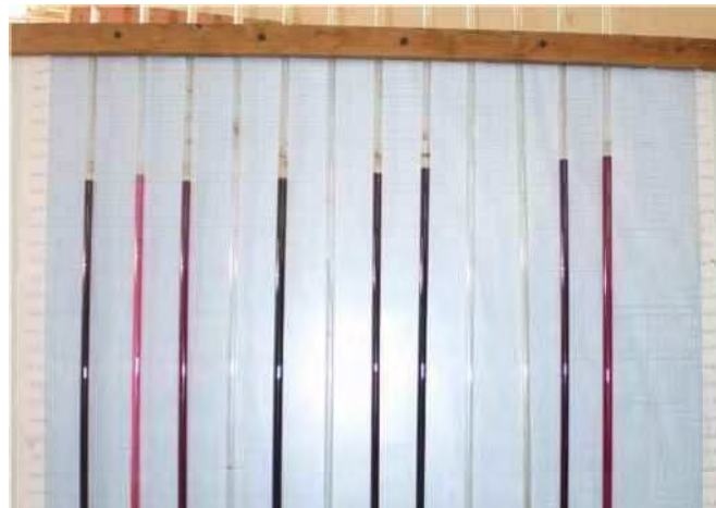
Plate (8) Piezometer Tubes Board for Measuring Pressure Distribution on the Sill and the Horizontal Apron
