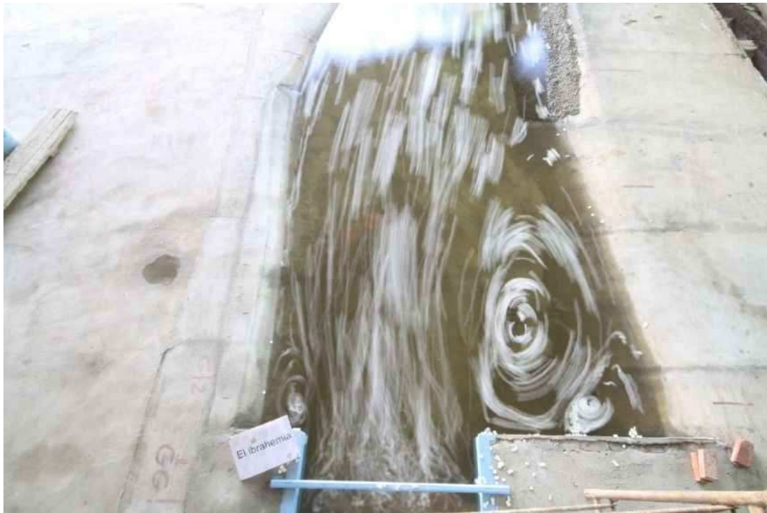
Photo 5: Flow Tracking Downstream New Ibrahimia Regulator Using Floating Debris
