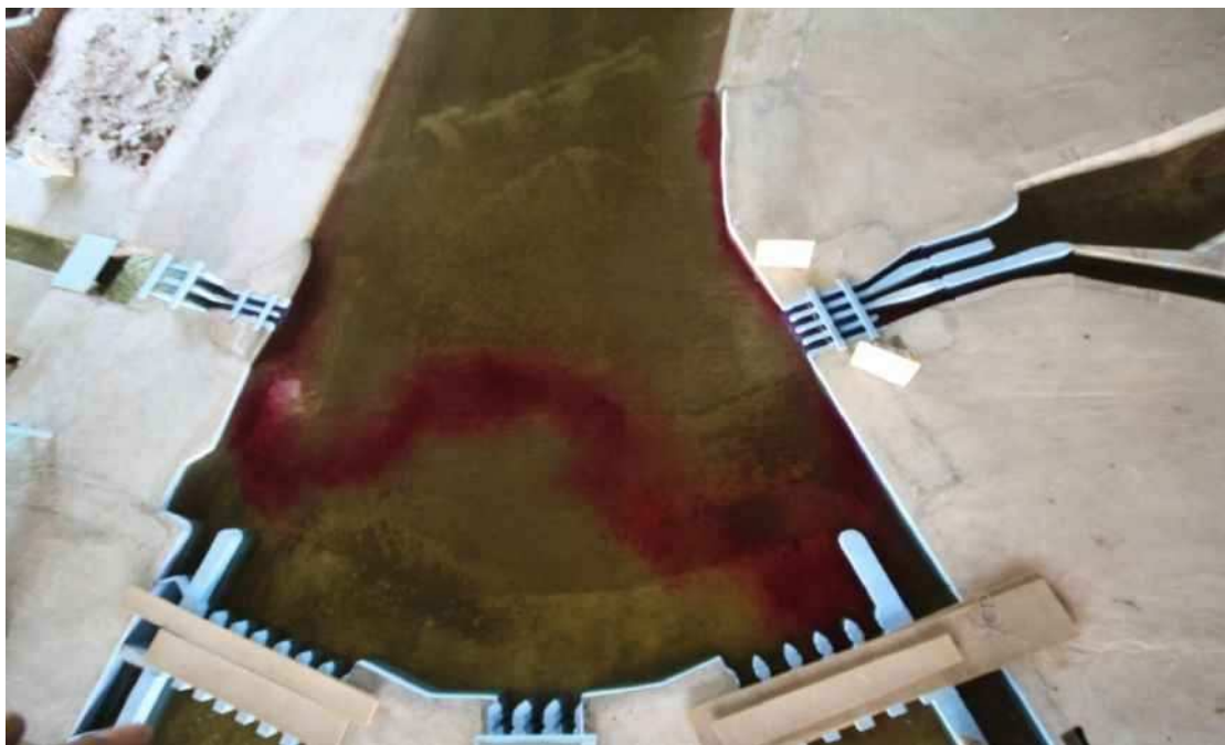
Photo 2 : Flow Tracking Upstream Existing DGRs Using Colored Dye
