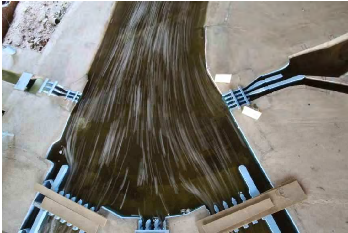
Photo 1: Flow Tracking Upstream Existing DGRs Using Floating Debris
