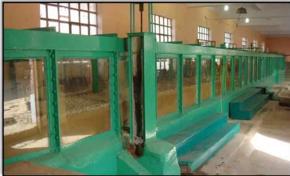
Plate (1) 2D Flume in the Hydraulic Laboratory of the Hydraulics Research Institute (HRI), Egypt
