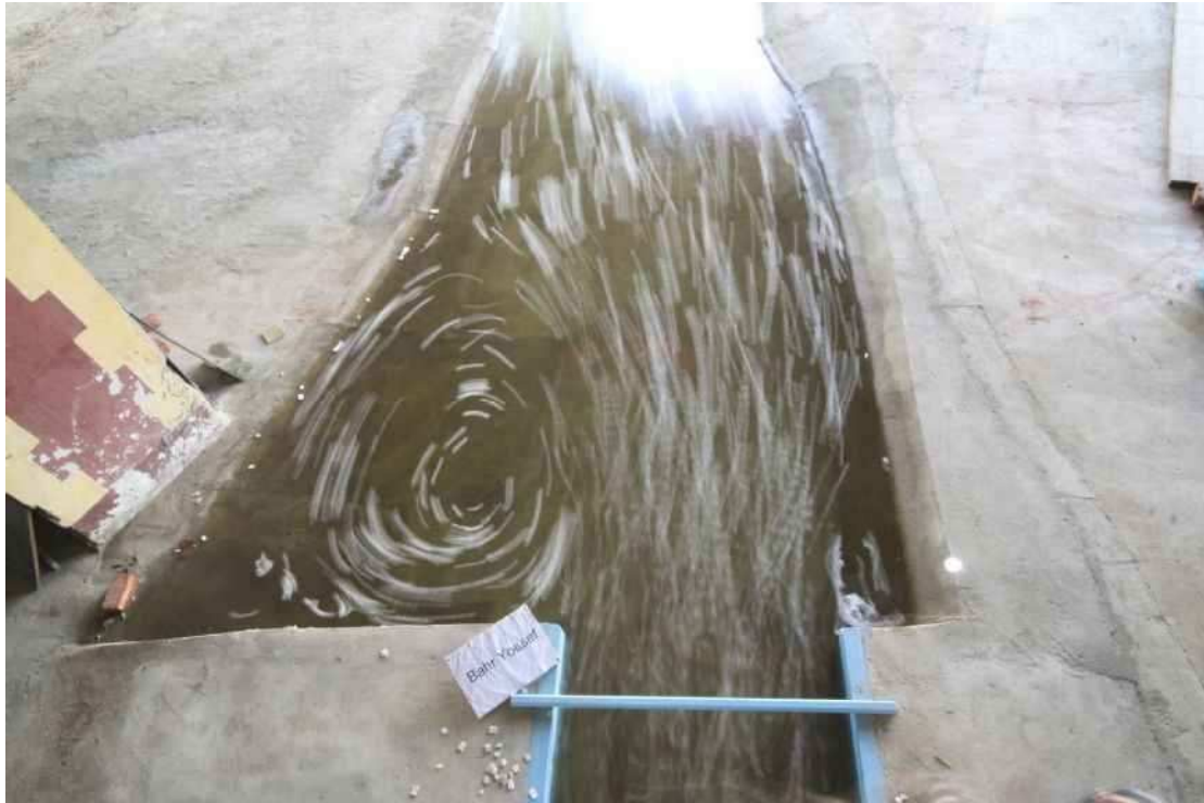
Photo 7: Flow Tracking Downstream New Bahr Yusef Regulator Using Floating Debris
