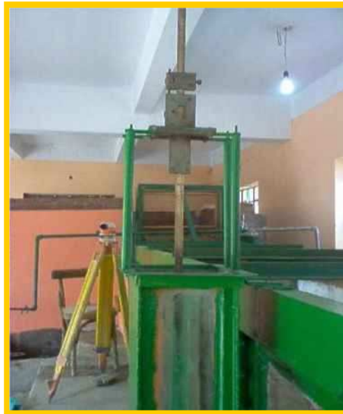
Plate (7) Point Gauge Device for Adjusting the Model Water level
