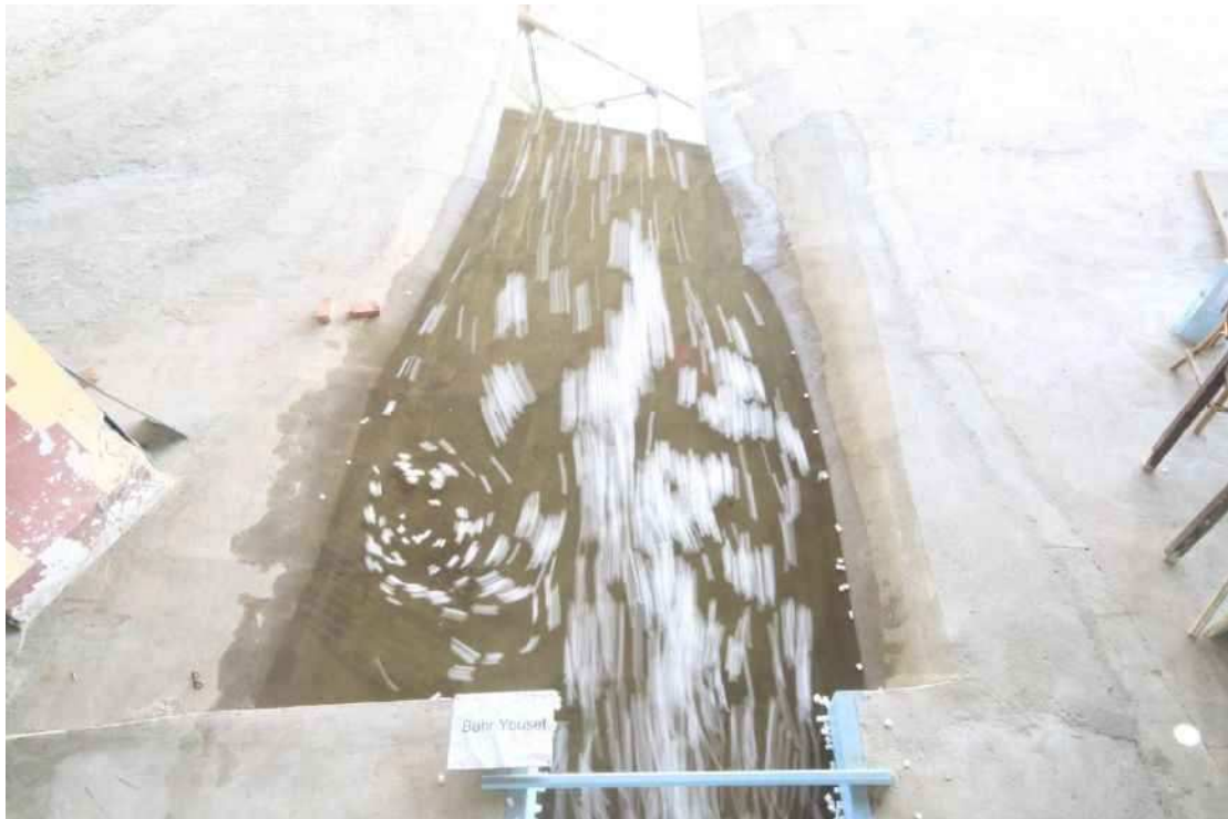
Photo 11: Flow Tracking Downstream New Bahr Yusef Regulator Using Floating Debris
