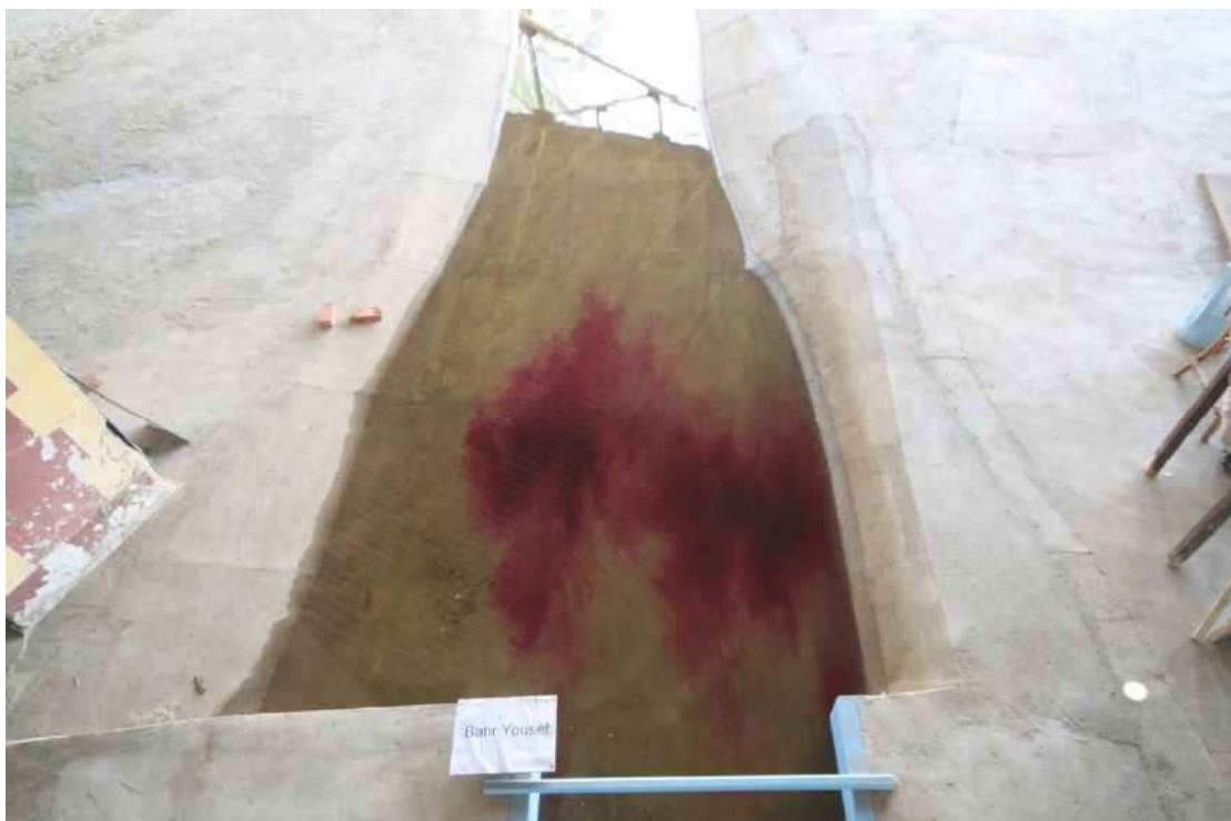
Photo 12: Flow Tracking Downstream New Bahr Yusef Regulator Using Colored Dye
