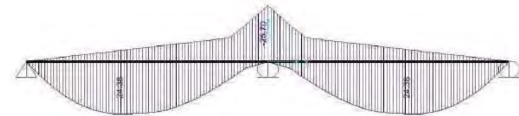
Maximum and minimum bending moment (Fatigue model)
