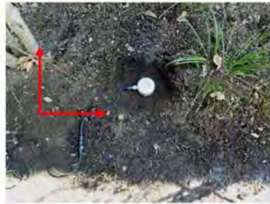
Setting a vibration pickup on the suitable measurement point along the boundary line
