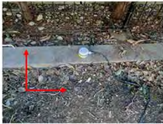
Setting a vibration pickup on the suitable measurement point along the boundary line
