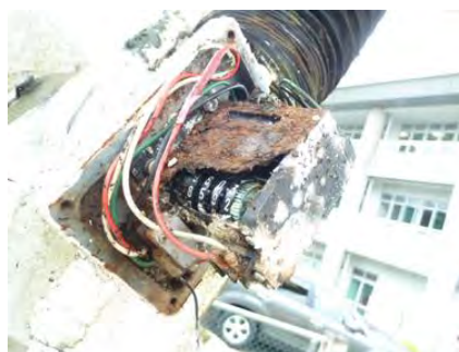
Picture 7: Damage to EL Resolver (elevation rotation angle detector) / Limit Switch Module (position detector)
