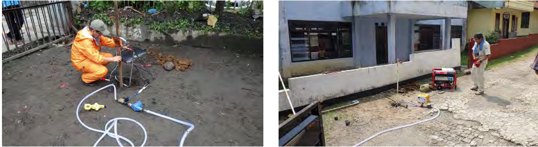
Photo 1 In-situ Permeability Test in BAPPEDA Office[left] and Kec. BOUT Office[right]
