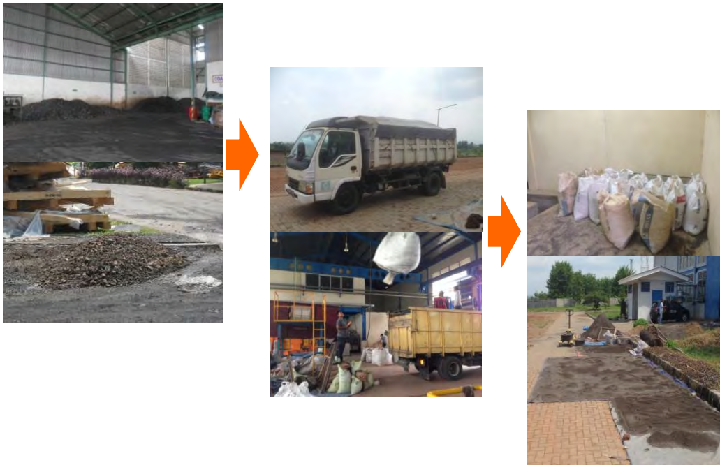
Figure2 Flow of coal ash handling
