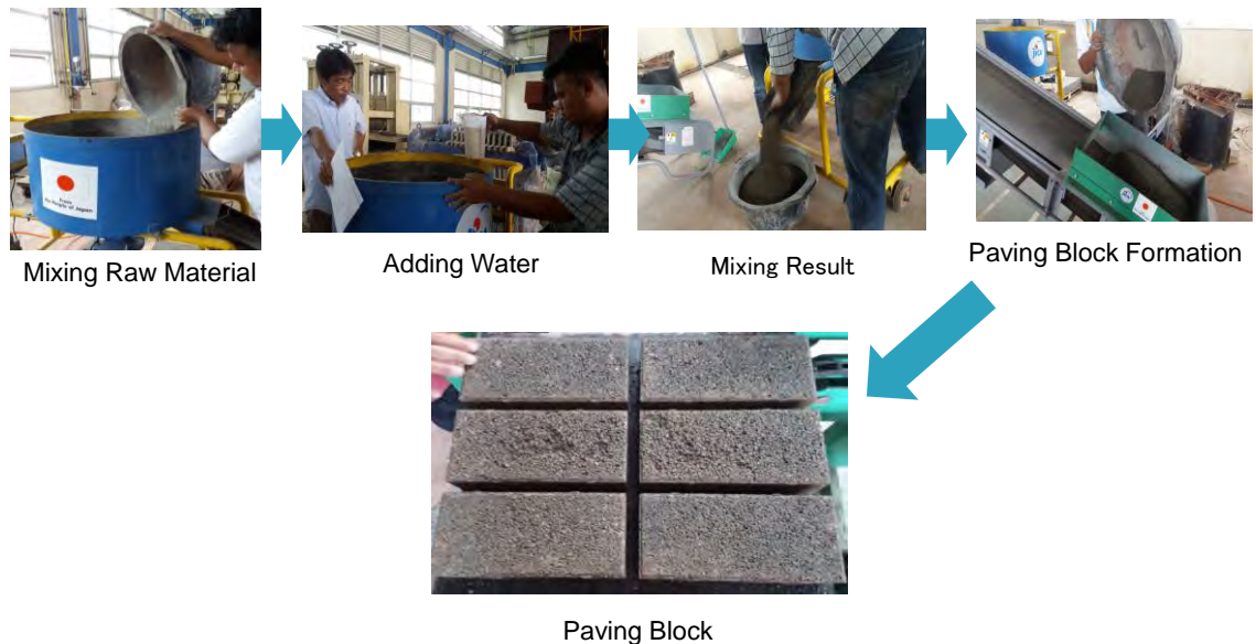
Figure4 Flow of the production of SLS blocks
