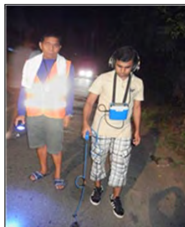
A trainee of CWASA (right) conducting mid-night leakage survey, with the assistance of a trainer of Metro Cebu WD (left) in Philippines.
