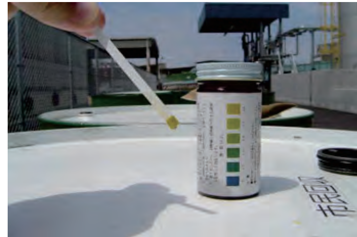
Checking Acid Value by color chart
