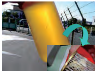
Unclear fuel (without additive)
