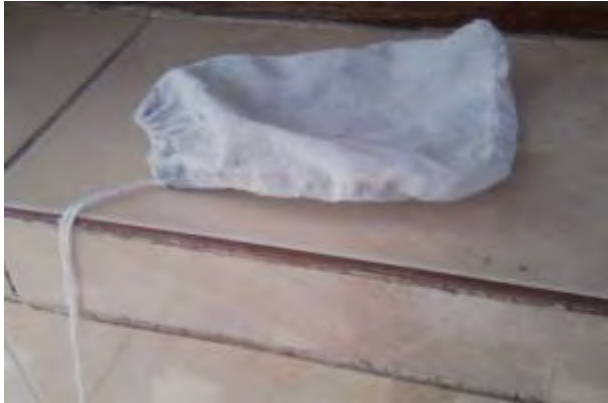
Cloth filter that was used until some years ago
