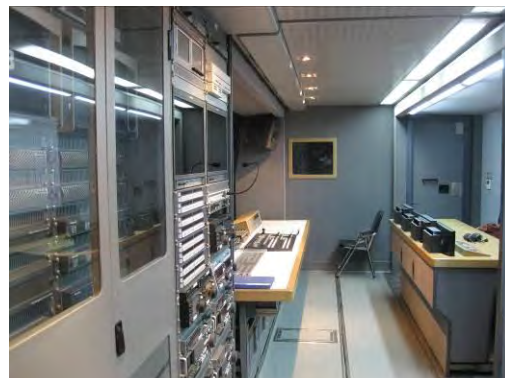
Inside of HDTV Broadcasting Van (QHBTV)
