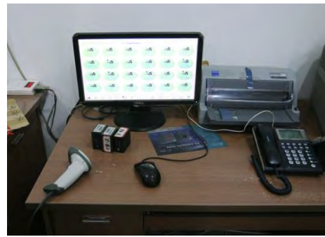
A bar-code reader system for management of usage of equipment
