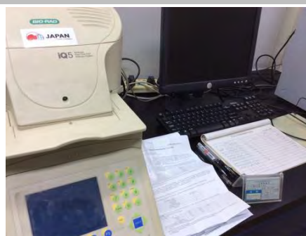
A device for genetic testing and the usage record. This device was most useful in examinations of viruses. (Henan Province CDC)
