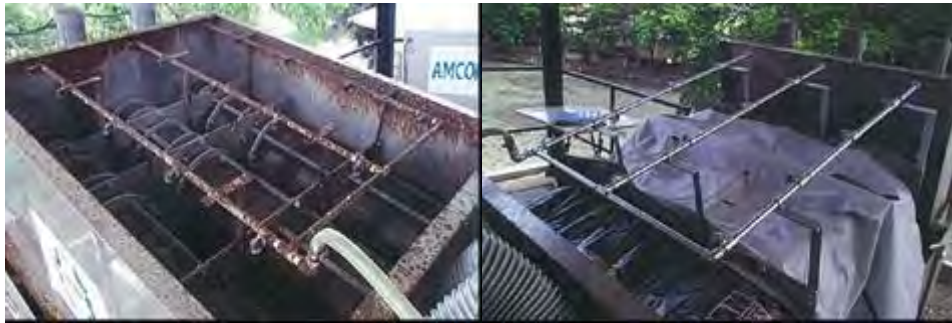
Photo: Dewatering press become rusty and after providing protection (Aug, 2014)
