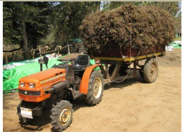
Small tractor is also one of target of government subsidy programme. This tractor is 24 horse-power and 4 wheels manufactured. (Vizianagaram District)
