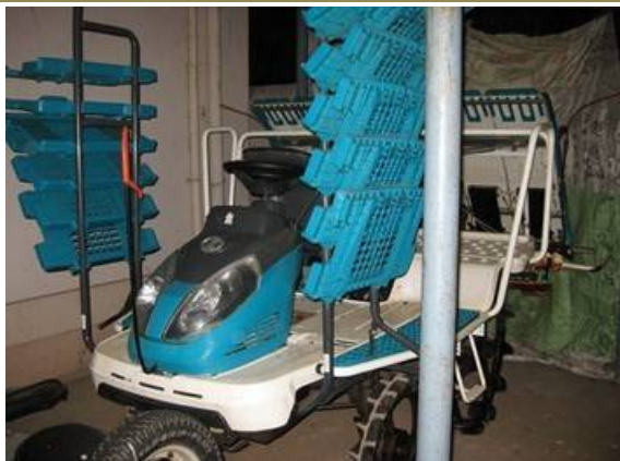
Rice transplanter is one of components of government subsidy programme. This transplanter is a model of 6 rows riding type. (West Godavari District)
