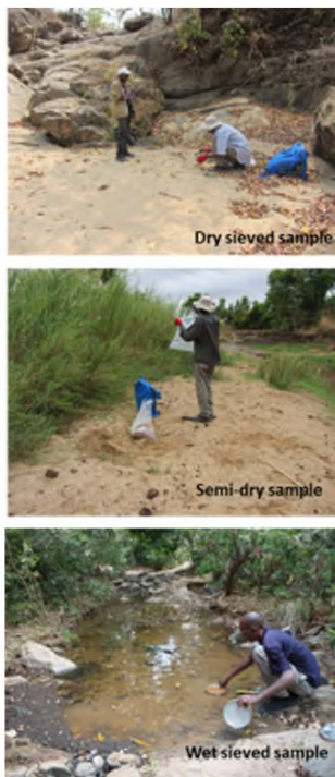
Photograph-18 Dry sieved / semi-dry / wet sieved sampling
