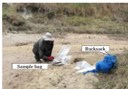
Photograph-17 Transcribing the site number onto sample bag by black marker pen
