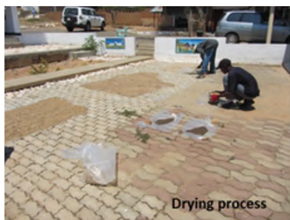
Figure 3-1 Sample drying and sieving in field base (Mzimba)
