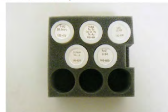
Figure 2. The Soil/Mining QC Reference Sample Set
