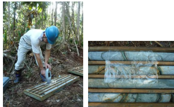
Figure-B: Plastic bag usage between sample and XRF
