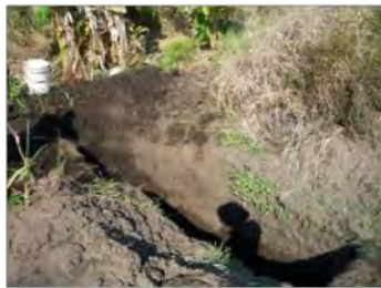
IS69: Black clayey soil (Dambo) of flood plain. [Cu: 74.2ppm, Co: 39.1ppm, Ni: 132ppm, Cr: 166ppm]
