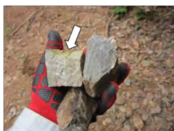
FT27: calcareous-siliceous gneiss with felsic vein and epidote-K-feldspar veinlet [Au: 0.133ppm, Cu: 17.6ppm]
