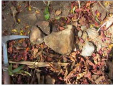
KT12: Dolerite fragment and magnetite rich sediments. Karoo dolerite and basalt with tuffaceous conglomerate with Mt, Py-Cpy (now limonitic) dissemination. [Cu: 61.5ppm, Co: 52.1ppm, Cr: 626ppm, Ni: 158.5ppm]
