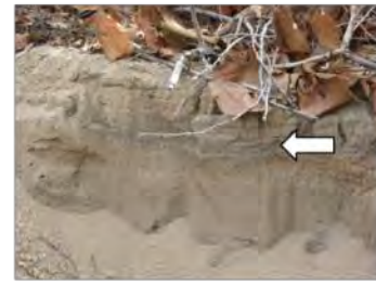
FT47: magnetite layers (black layers, probably with zircon) in stream sediments [Zr: over 500ppm, Ti: 6.69%]
