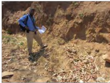
AT02: Alluvial terrace creek. Sheared syenite, pegmatite and laterite fragment contained sediments. [Nb+Ta:427.3ppm, Ti:4.48%]
