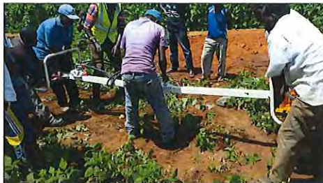
Setting ink needles for the base of the penetrometer
