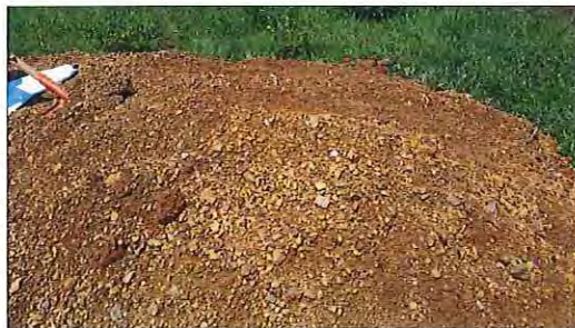
Earth excavation encountered scattered pebbles from 3.40 m deep
