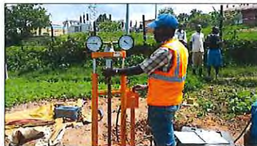
Penetrometer in action : measuring applied forces
