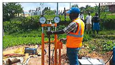
Penetrometer in action : measuring applied forces
