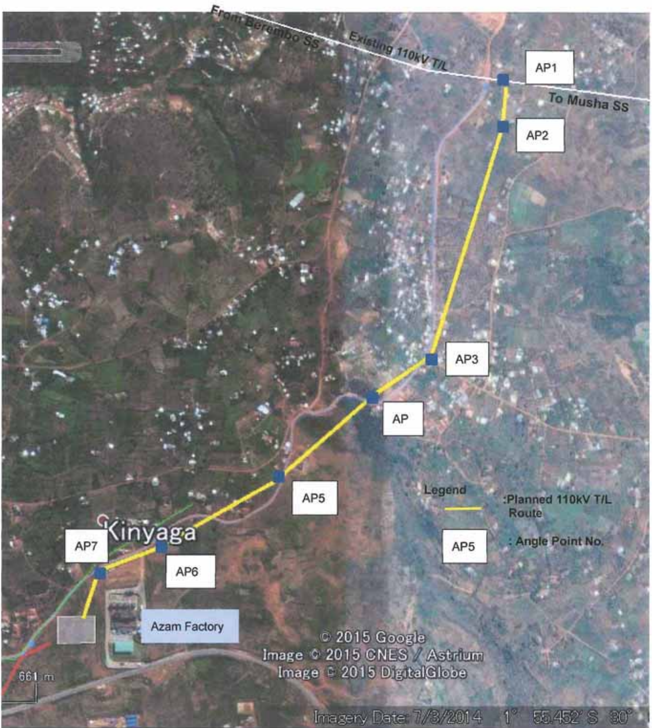
DWG No. TL01: Plan Drawing for 110kV Transmission Line
