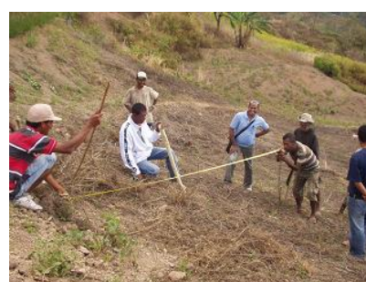
A one-meter stick should be used to check the vertical distance between contour lines.
