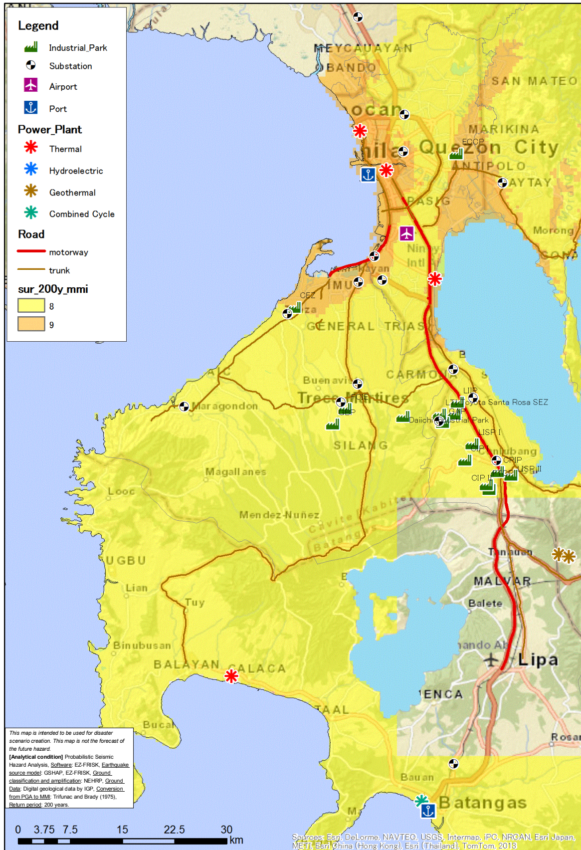
Figure 5.2 Seismic Intensity for the probability of a once in 200 years Earthquake (Cavite, Laguna, and the Southern Part of Metropolitan Manila in the Philippines)
