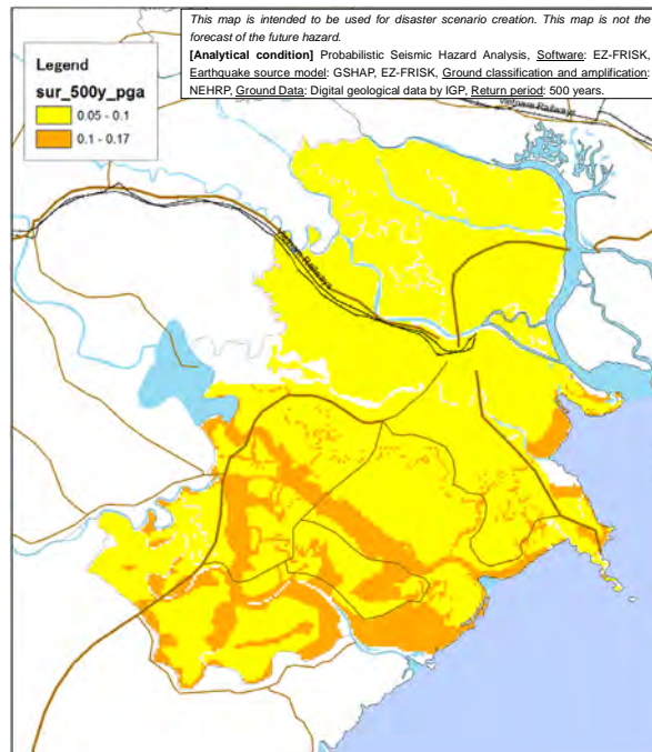
Figure A.1.11 Surface acceleration distribution (expected for 500 years, unit: g)
