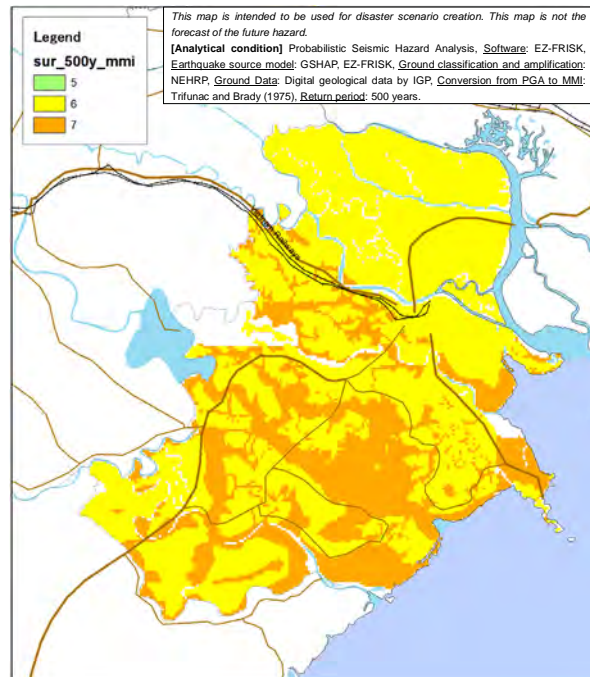
Figure A.1.15 Seismic intensity distribution (expected for 500 years in MMI scale)
