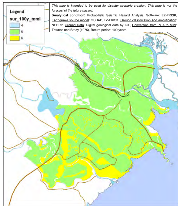
Figure A.1.13 Seismic intensity distribution (expected for 100 years in MMI scale)
