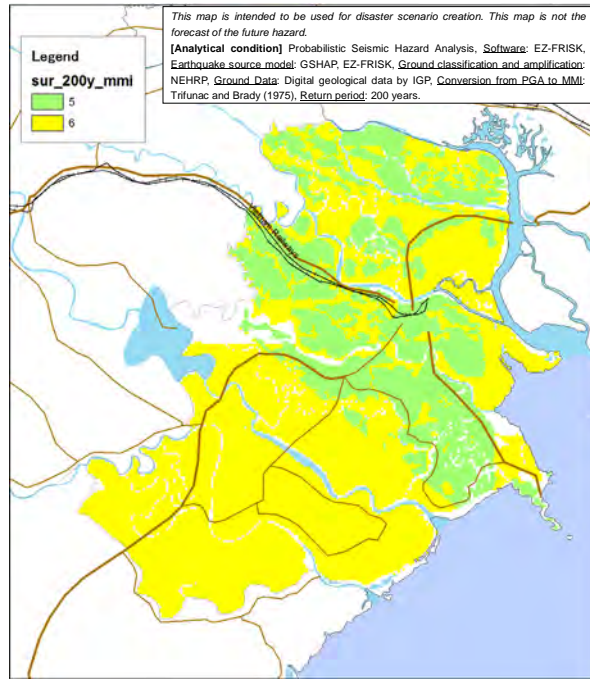
Figure A.1.14 Seismic intensity distribution (expected for 200 years in MMI scale)
