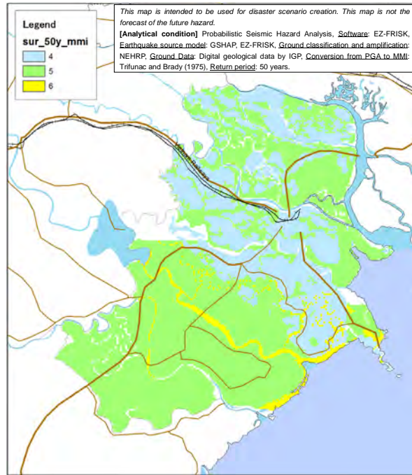
Figure A.1.12 Seismic intensity distribution (expected for 50 years in MMI scale)
