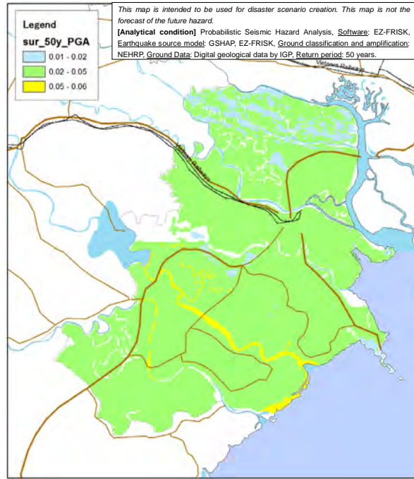
Figure A.1.8 Surface acceleration distribution (expected for 50 years, unit: g)
