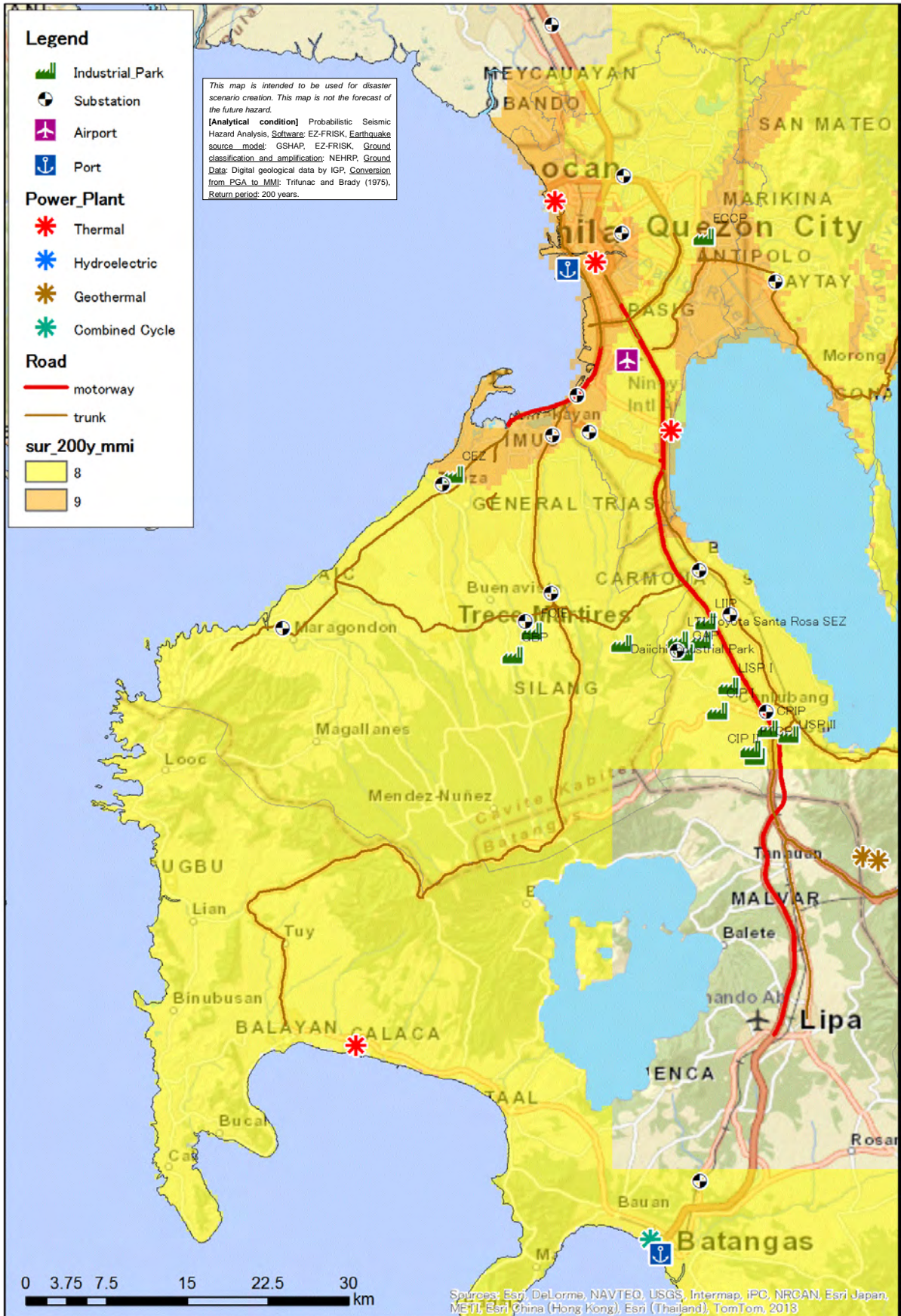
Figure 1.2.2 Seismic intensity expected with a 200-year probability and the distribution of important facilities
