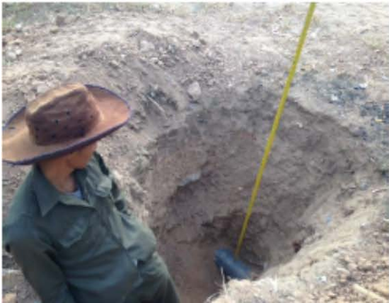
Test Pit No.18 (Gray Color 200PVC Pipe Found) Pipe Found)
