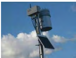
Components of Weather Station
