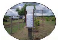
Type of rain gauges that are used for community Flood early warning
