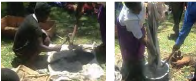
Step 3: Crush the heated wastes into dust and mix it with adhesive fluid
