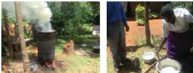
Step 2: Heat the agricultural waste using the kiln and prepare adhesive
