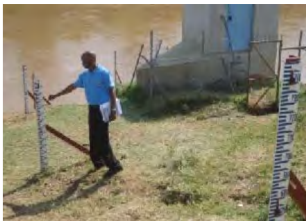
The e river gauging at Wath Ongor that the WRUA members used to gather data and developed the Hydro-graph that they can use for early warning during floods disaster
