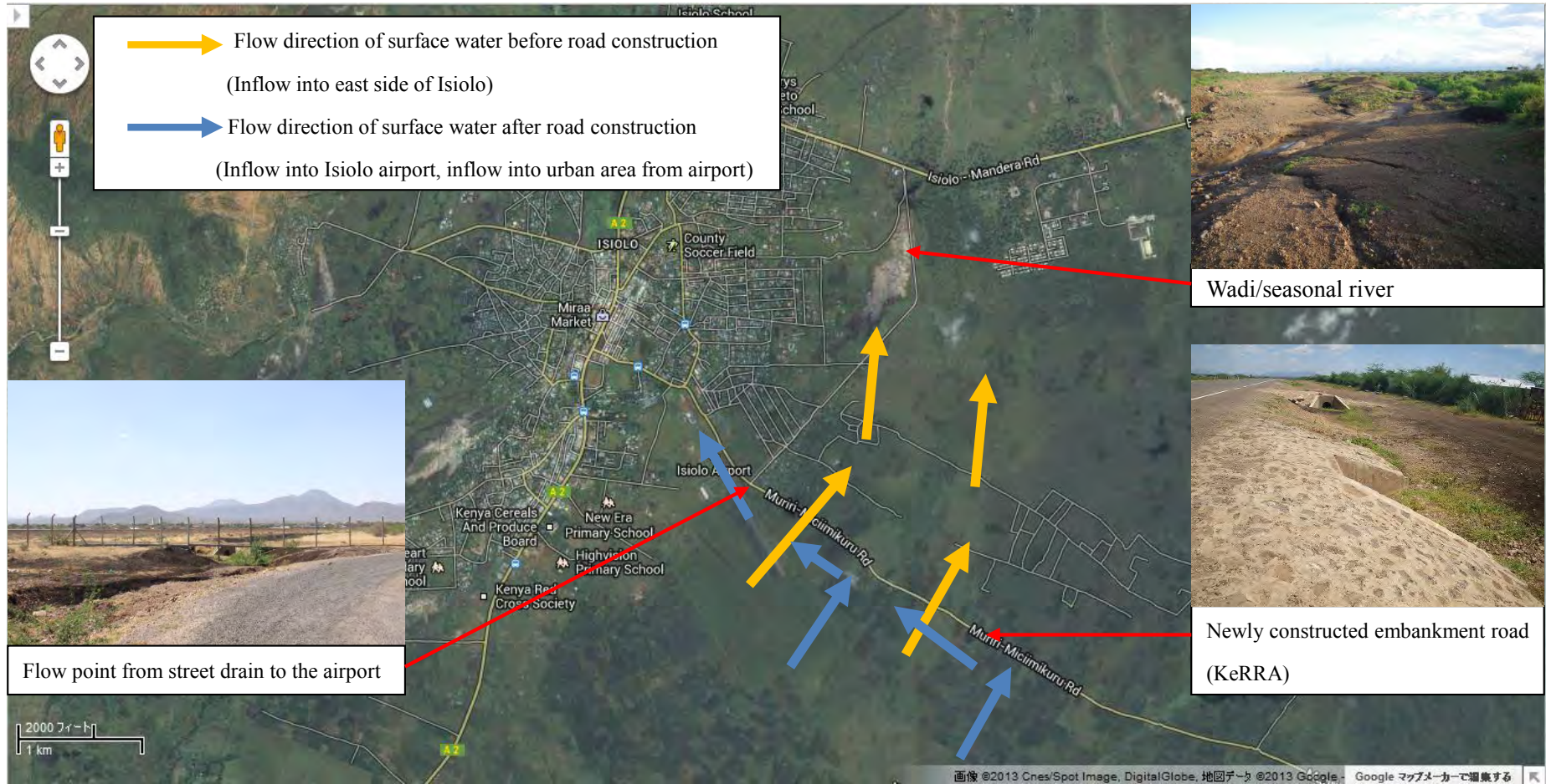
Figure 2.2.3 Direction of Rain Water from Airport Area
