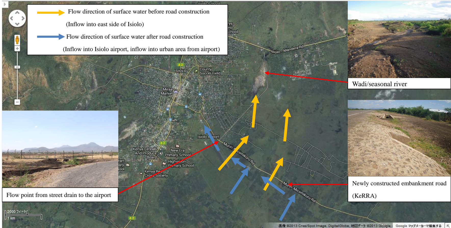
Figure 3.2.3 Direction of Rain Water from Airport Area
