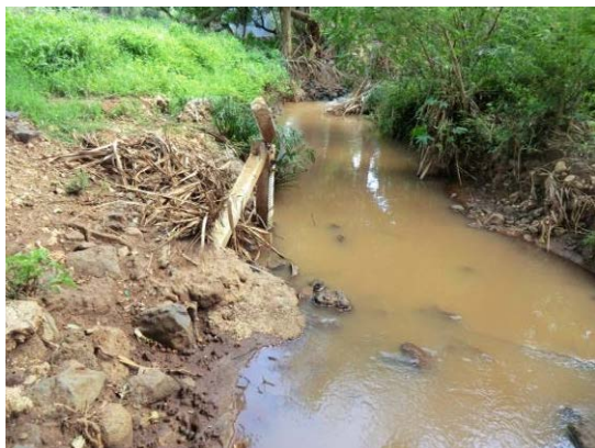
Water Level Gauging Station No.:5DA04 Observation River : Eastern Marania River Special Note : Water level gauge is broken off and damaged.
