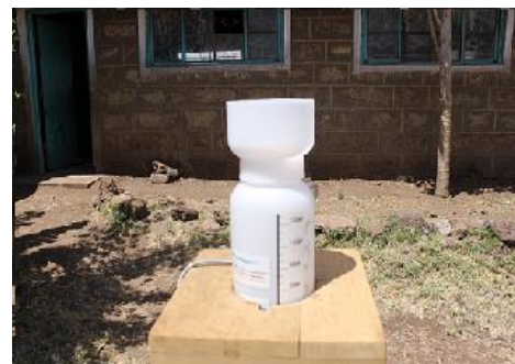
Simple Rain Gauge (Place: Nkando Primary School)
