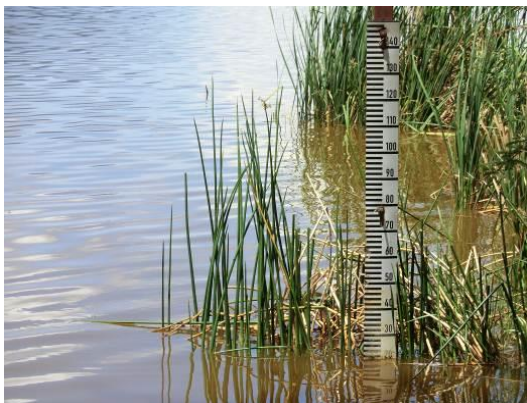
Water Level Gauging Station No.:3J2 Water level gauging station inside Safari Camp for measurement of water level of Lake Jipe
