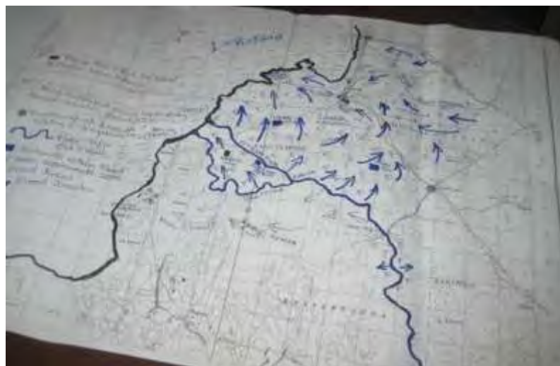
Marking out the flood water flow direction
