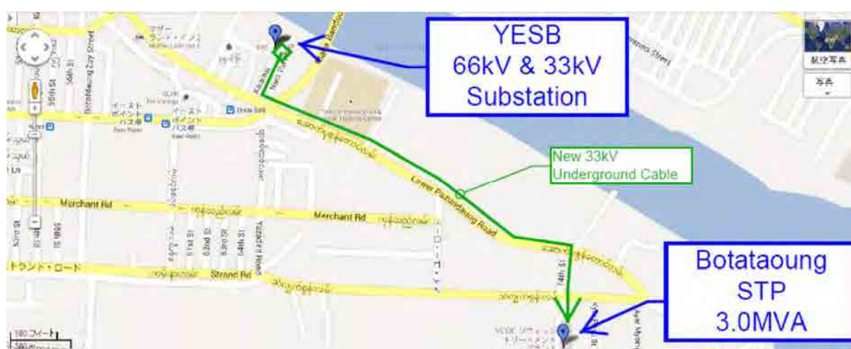
Figure 3.13 Wastewater Treatment Plant (WWTP) and 33 kV Underground Cable Route
