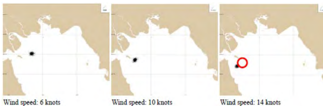
Figure 1.3-1(2) Trajectory of the spilled oil after 5 days in the closed-off the Persian Gulf (Season: Nov-Jan, Wind direction: Northeast)
