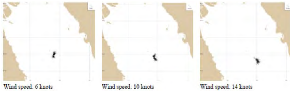
Figure 1.3-5(1) Trajectory of the spilled oil after 5 days at Foroozan oil field (Season: Feb-Oct, Wind direction: Northwest)
