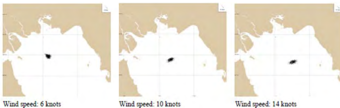
Figure 1.3-1(1) Trajectory of the spilled oil after 5 days in the closed-off the Persian Gulf (Season: Feb-Oct, Wind direction: Northwest)
