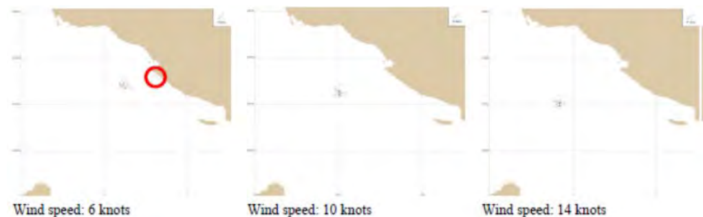
Figure 1.3-8(2) Trajectory of the spilled oil after 5 days at the SPM system at offshore for loading of condensate, Assaluyeh (Season: Nov-Jan, Wind direction: Northeast)
