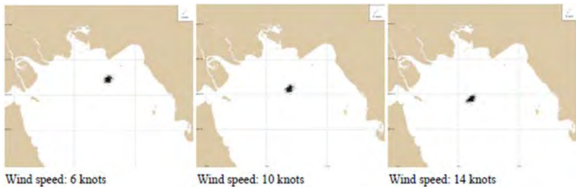
Figure 1.3-2(2) Trajectory of the spilled oil after 5 days at Bahrgan Sar oil field (Season: Nov-Jan, Wind direction: Northeast)
