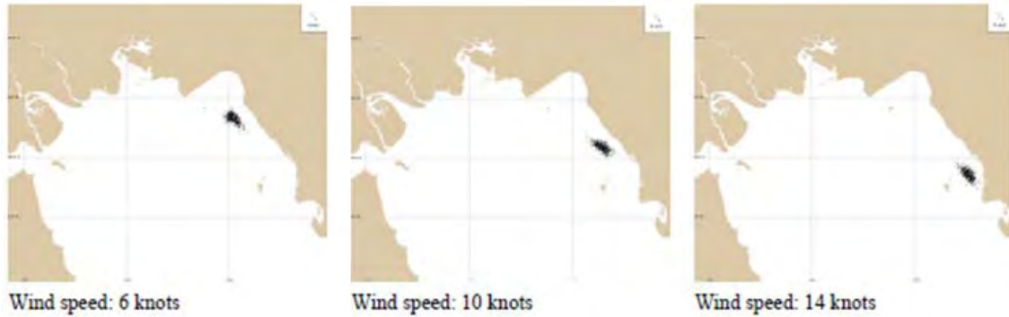
Figure 1.3-1(1) Trajectory of the spilled oil after 5 days at Bahrgan Sar oil field (Season: Feb-Oct, Wind direction: Northwest)
