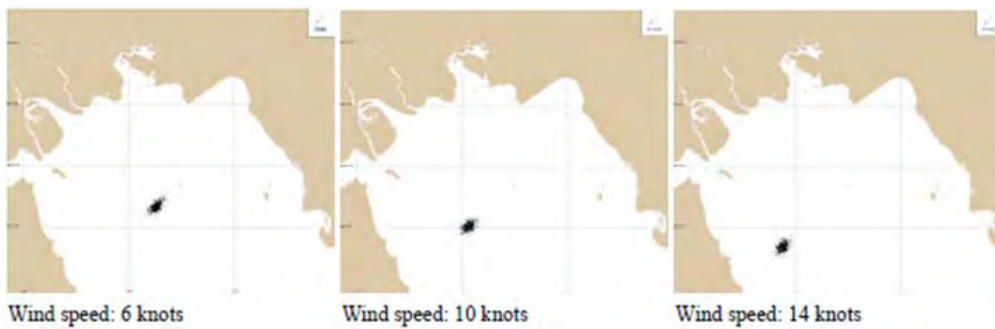
Figure 1.3-4(2) Trajectory of the spilled oil after 5 days at Aboozar oil field (Season: Nov-Jan, Wind direction: Northeast)
