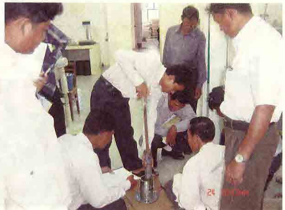
Practice on soil compaction test
