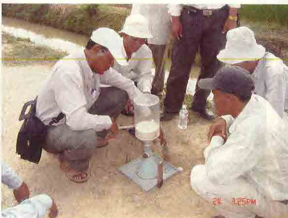
Practice on field density test
