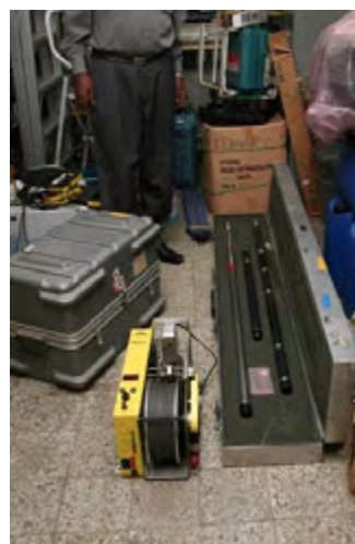
Well logging machine and probe (small generator is needed to operate)
