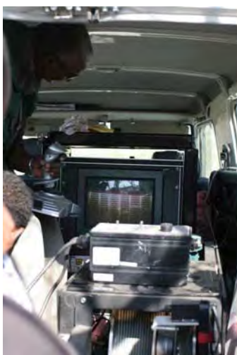
Practical training of bore hole camera (monitor and winch are used from within vehicle)
