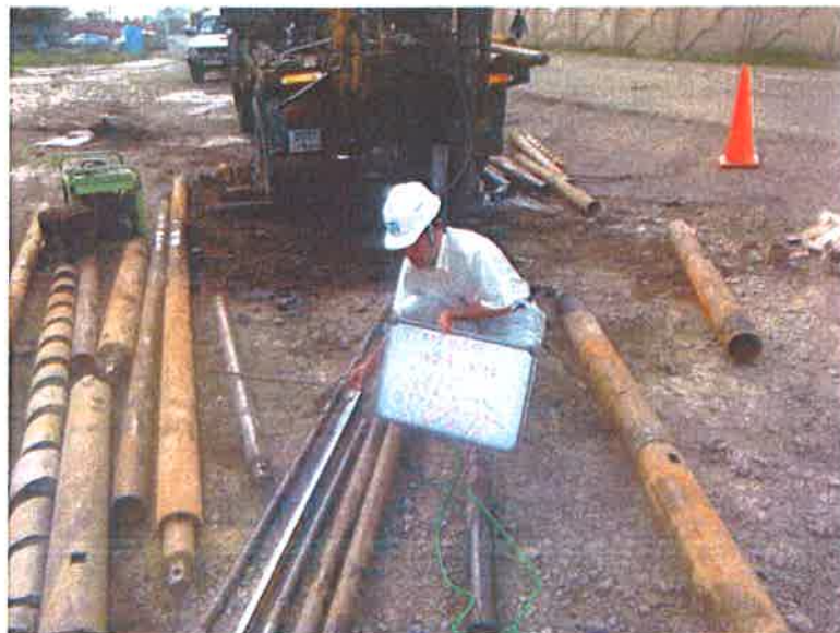
Photo-6 Certification the length of S.P.T No.6 L=16.0m
