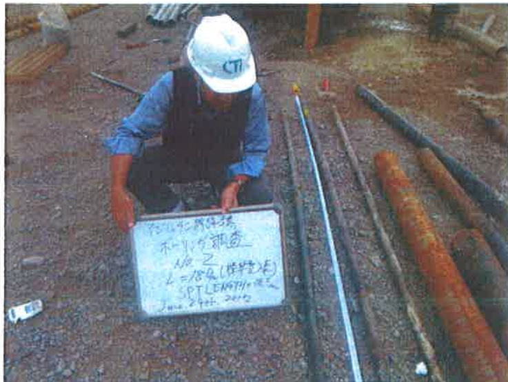
Photo-2 Certification the length of S.P.T No.2 L=18.0m
