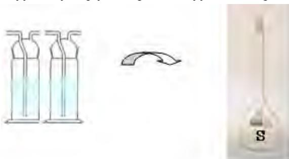
Fill the flask up to 250 ml gauge line
